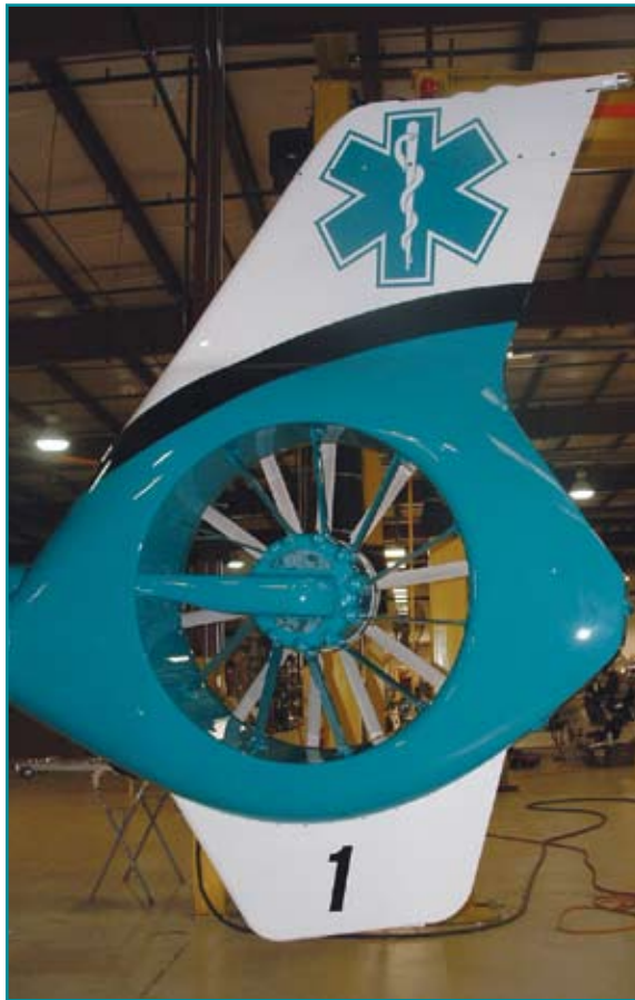
ABOVE: The EC135 features an enclosed Fenestron tail rotor allowing for safer operations.
